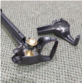
Remove crank case cover.
