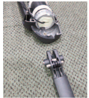
Remove steering rod from tilt degree mechanism.
