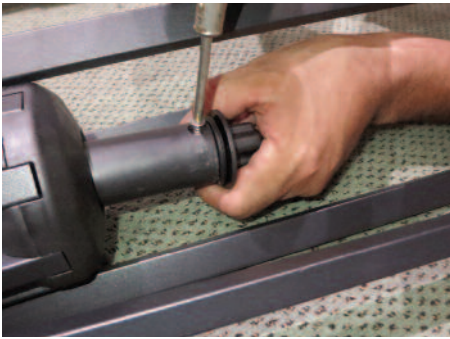
Pull down light adapter and remove cap and 2 screws using a Phillips screwdriver.
