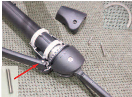
Insert support strut into tilt degree mechanism and secure with pin . Place top cover and retainer onto tilt degree mechanism and tighten with 4mm hexagon wrench.
