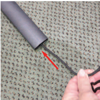
Guide cord end of steering rod.
