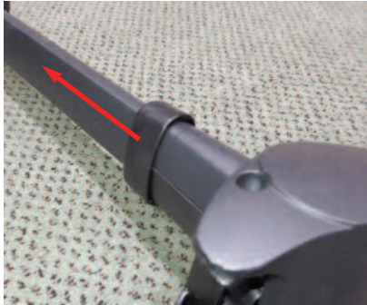
Slide ring off crank case and down steering rod.
