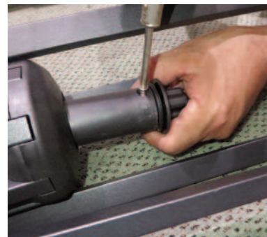
Reattach light adapter cap and secure with 2 screws.
