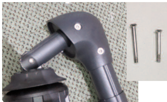
Reattach other side of hinge cover and secure with 2 bolts.
