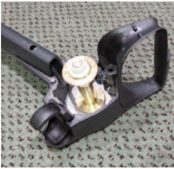
Reinsert steering rod into crank case.
