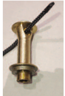
Insert new cord through smaller side of brass part.
