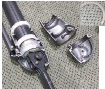
Remove 2 covers and retainer from tilt degree mechanism.
