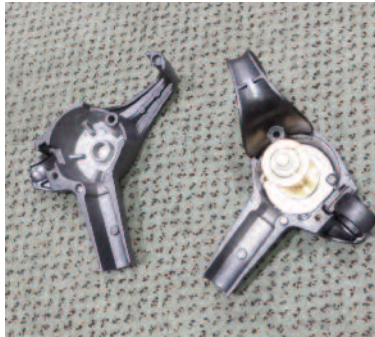
Remove steering rod from crank case and set aside.
