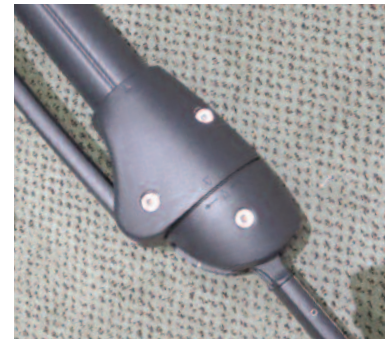
Place lower cover onto tilt degree mechanism and tighten with 2 bolts using 4mm hexagon wrench.
