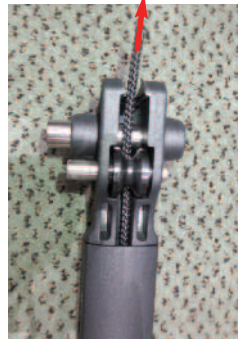
Pull cord through ??? end of steering rod.
