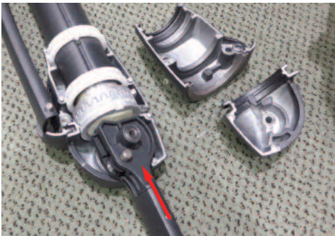
Place rod back into tilt lever mechanism by pushing up into tilt degree mechanism.
