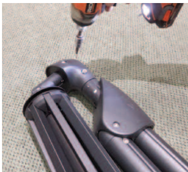
Remove 2 bolts from hinge.
