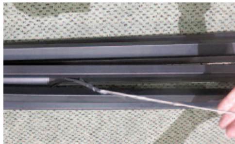
Pull rod with taped cord through lower runner. Set aside.
