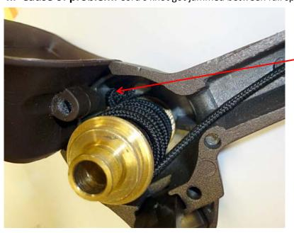
Knot got jammed between spool of cord and housing. This can happen only when the umbrella is fully opened.
