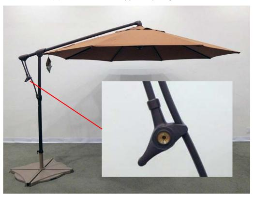
II. Cause of problem: Cord's knot got jammed between full spool of cord and crank housing.
