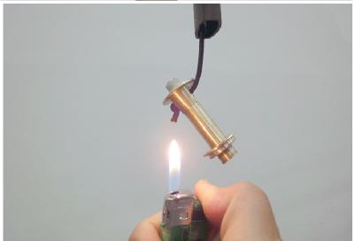
Cut off unneeded cord below the new knot and partially melt the cord end to prevent fraying.
